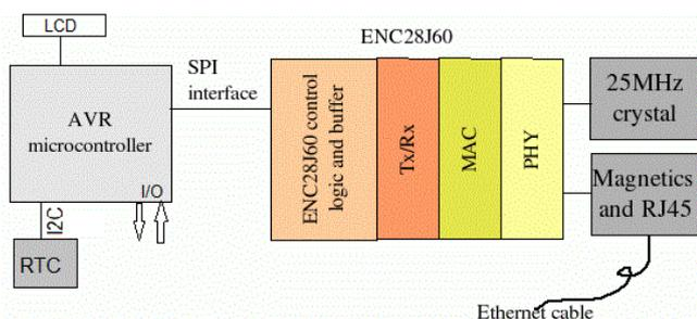
Fig 1. The hardware architecture a web home controller
